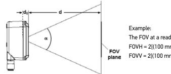
The FOV at a reading distance of 100 mm is:
